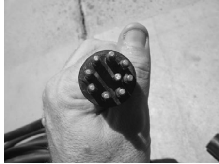
Male eight-pin connector with stainless steel locator pin.
